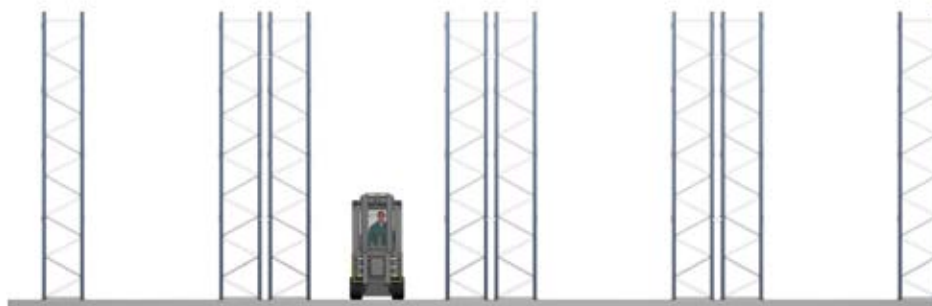
The most common conventional system comprises a single-entry rack fitted to the wall and double-entry racks in the middle
