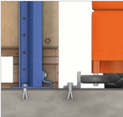
Guidance using LPN 50 profiles The pallets are set directly on the floor.
